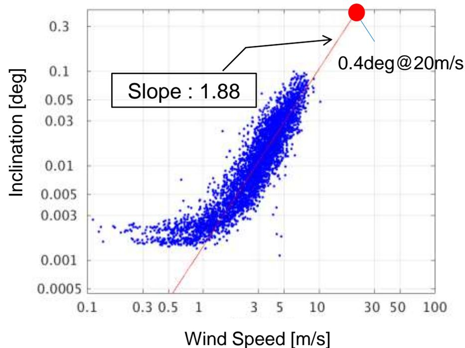
Distribution of Wind speed vs. Inclination
