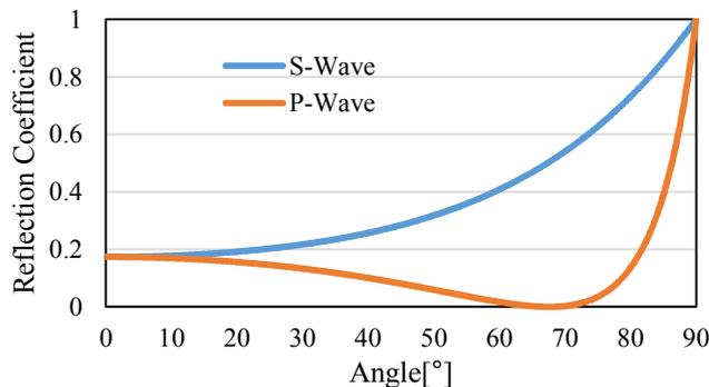
Fig. 8 Reflection coefficient of concrete
