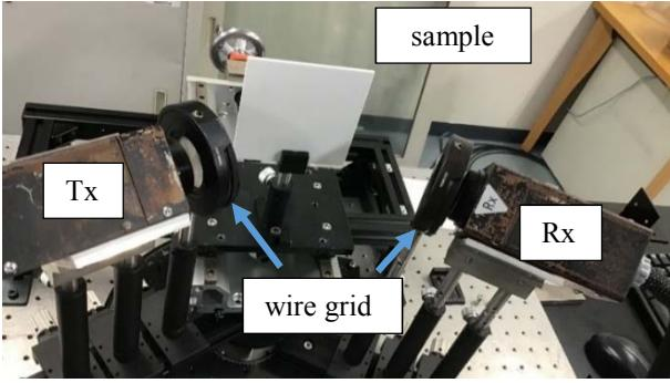
Fig. 2 Photograph experimental setup of THz-TDS
