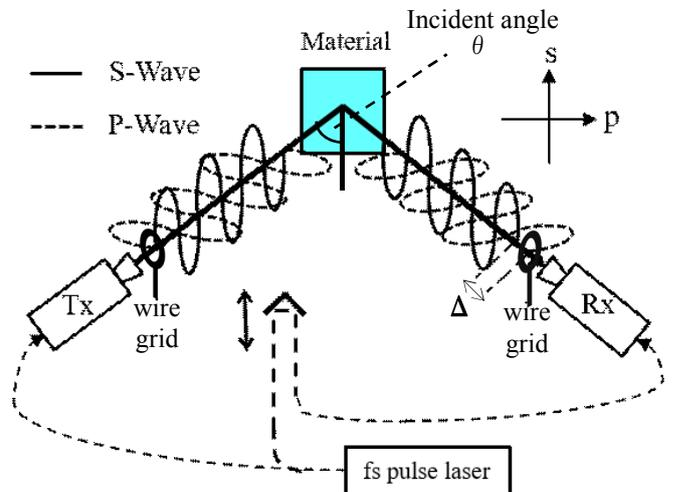
Fig. 1 Experimental setup of THz-TDS
