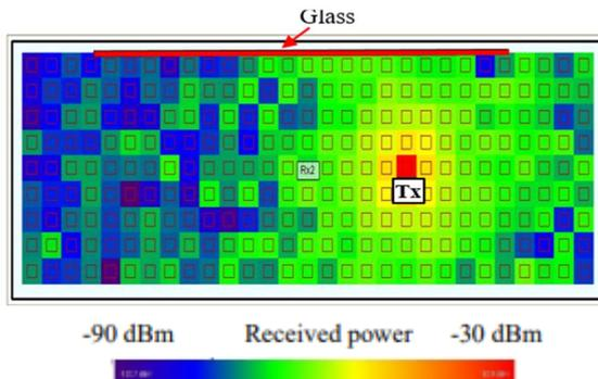
Fig. 12 Simulation results of received power map that employs ITU-R material property models [5].
