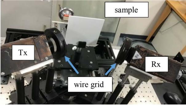
Fig. 2 Photograph experimental setup of THz-TDS
