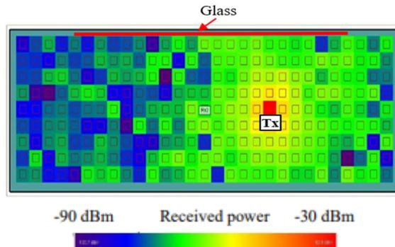
Fig. 11 Simulation results of received power map that employs our material property models.
