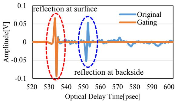
Fig. 5 The pulse waveform of a plastic sample.
