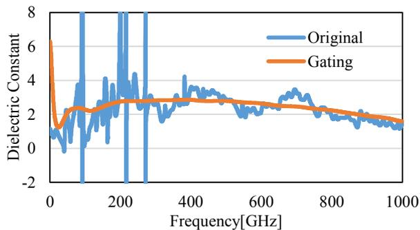
Fig. 6 Real part of plastic complex permittivity calculated from the pulse waveform with and without time-gating
