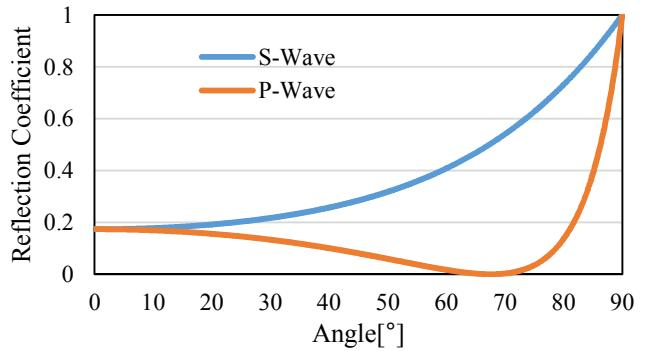
Fig. 8 Reflection coefficient of concrete
