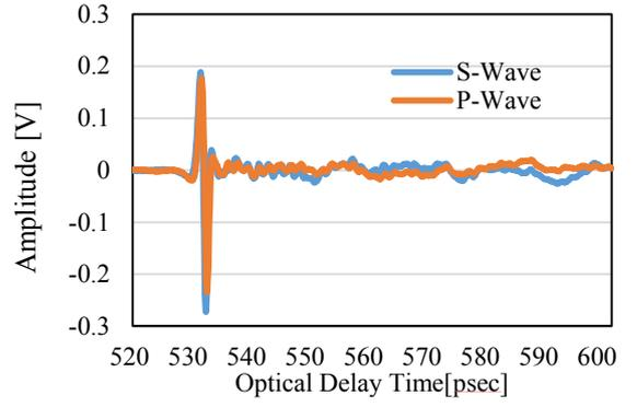
Fig. 3 Time waveform of the THz-TDS pulse signal that was reflected by metal with an incident angle of  $60^\circ$ .
