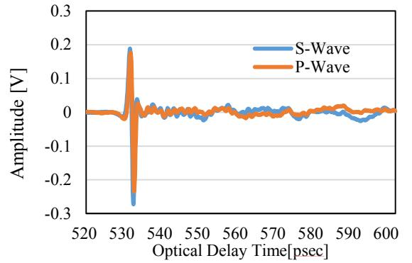
Fig. 3 Time waveform of the THz-TDS pulse signal that was reflected by metal with an incident angle of 60°.
