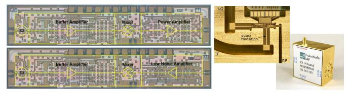
Fig. 7: Chip photos of the transmitter (top) and receiver (bottom) MMICs packaged in a split-block waveguide module (right).
