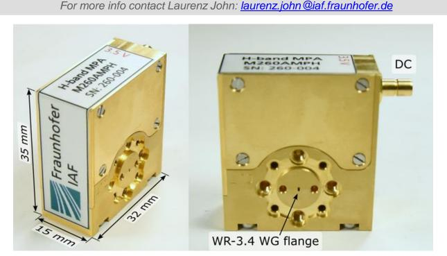
Fig. 6: Photographs of the developed WR-3.4 300 GHz solid-state power amplifier.
