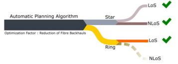
The algorithms try to find an optimum solution for the backhaul network. The optimisation factor of the developed algorithms is set as the reduction of cable connections, so the optimum solution is a backhaul network with potentially many wireless links instead of fibre connections. The search
