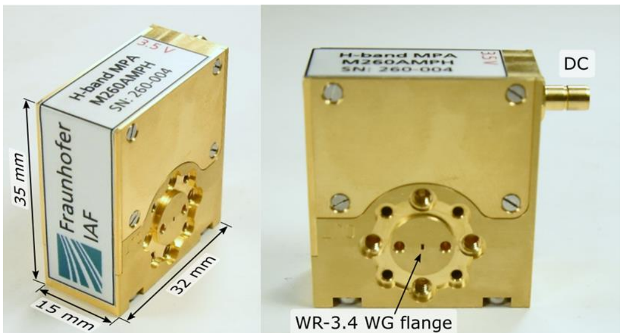
Fig. 6: Photographs of the developed WR-3.4 300 GHz solid-state power amplifier.
