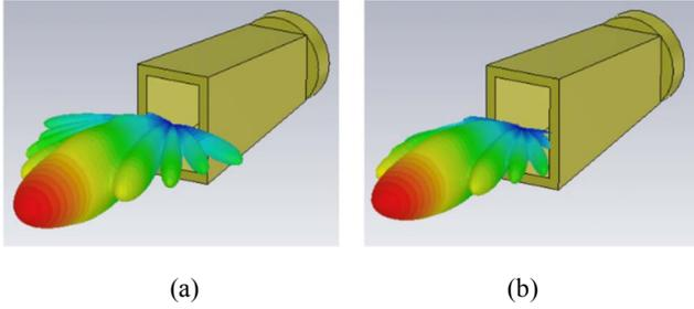
Fig. 6 Far-field pattern. (a) Simulation, (b) calculated from measured near-field pattern. The horn antenna in this figure is the polygon data used in the simulation, i.e., the 3D simulation model and the experimental results are put together to show the radiation characteristics.
