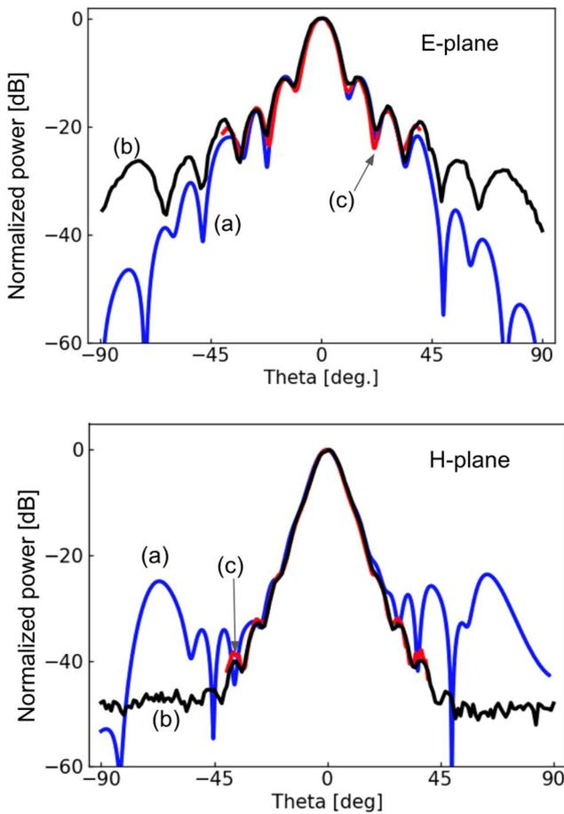
Fig. 5 Experimentally obtained far-field pattern. (a) Calculated from near-field pattern measured by EO sensing (blue), (b) conventional far-field measurement with spherical scanning (black), (c) conventional far-field measurement with planar scanning (red).
