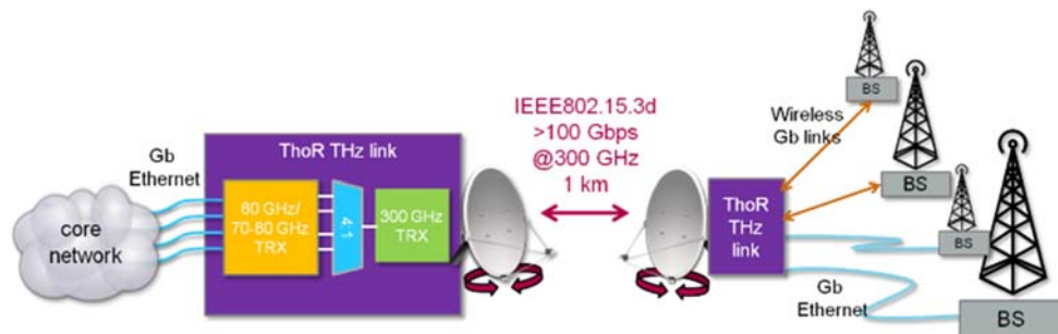
Fig. 1. ThoR wireless transport link integration in a live network, as the first use of THz frequencies in an operational network.
