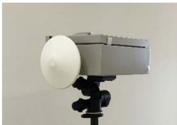
Fig. 7.3: Photograph of 300 GHz-band transmitter.
